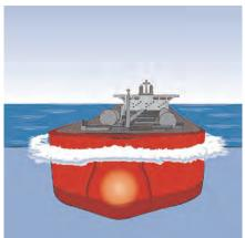
Large ships at maximum draft have minimal under keel clearance and can only manoeuvre within the designated shipping channel.
