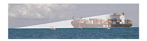
Large ships with the bridge at the stern will have a large blind spot for several hundred metres in front of the bow. This blind spot extends much further forward if deck cargo or containers are carried.
